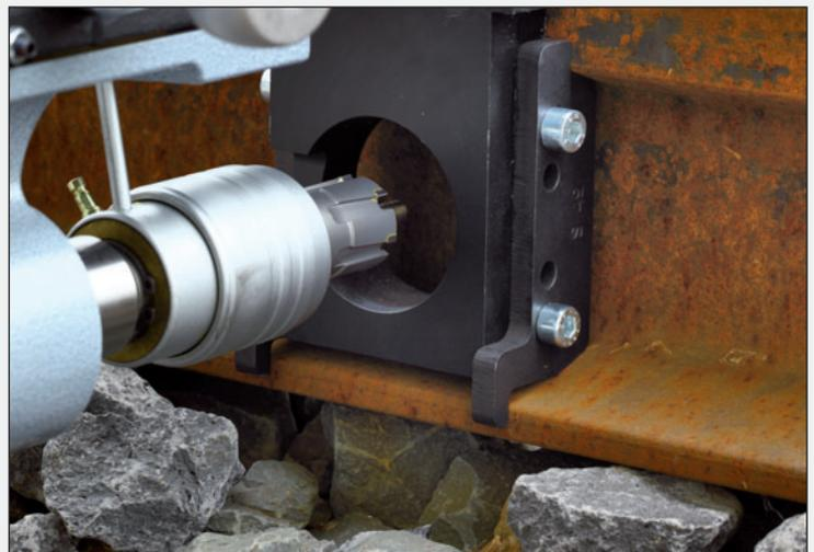
EJECTOR PIN FOR HKK-R, Ø 17 - 36 mm
